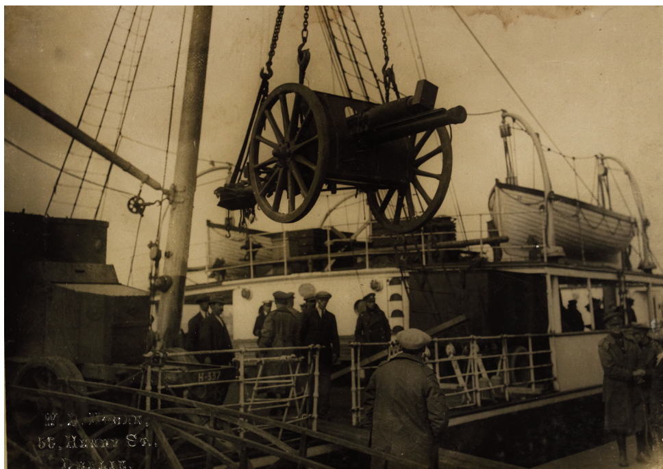
Left: Fig. 2—A Mark I 18-pounder (note the distinctive tank fitted to the recoil system above the barrel) being unloaded at Passage West from the Lady Wicklow (courtesy of the National Library of Ireland).
