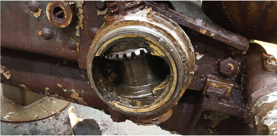
Left: Fig. 7—The 18-pounder's elevation gearbox with cover removed. Some of the original grease is still inside. The poor condition of the gun is very apparent.
