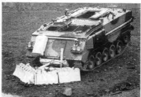
Pearson Engineering have developed a version of the Mine Plough with a hydraulically operated augmented blade. It is designed to sweep mines out of hollows and undergrowth where they might be undisturbed using conventional mine ploughs.
